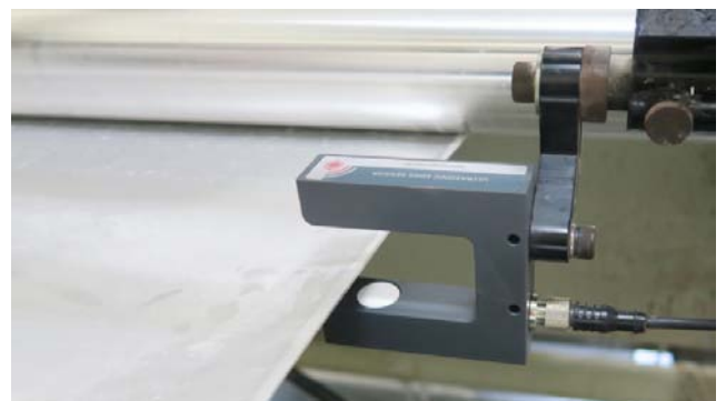
Ultrasonic Sensor DU-3 is used on aluminum foil
